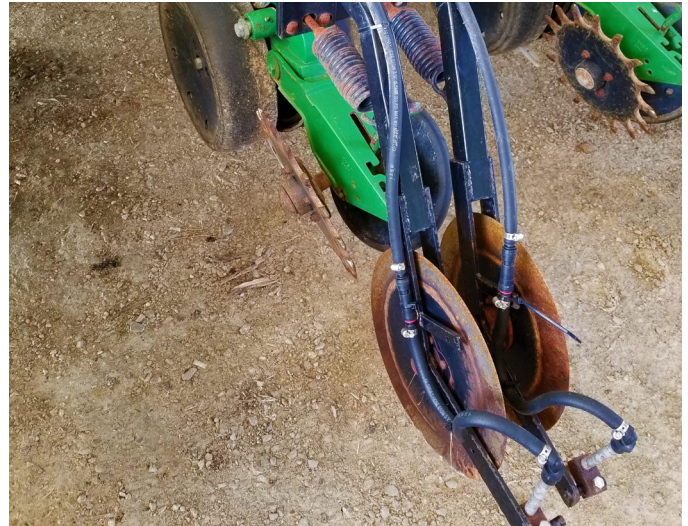
Figure 2. Starter fertilizer application system on row planter.
